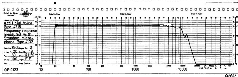
Fig. 3. Typical pressure response curve of the Artificial Voice with regulating microphone employed.
