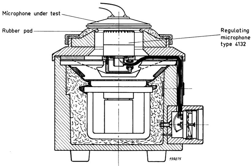
*Fig. 2. Artificial Voice with regulating microphone and test object mounted for pressure calibration.*
