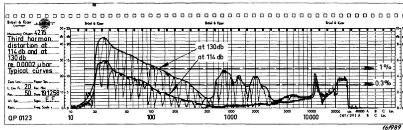
Fig. 11. Distortion generated in the Artificial Voice at sound pressures of 1 mbar and 0.1 mbar.
