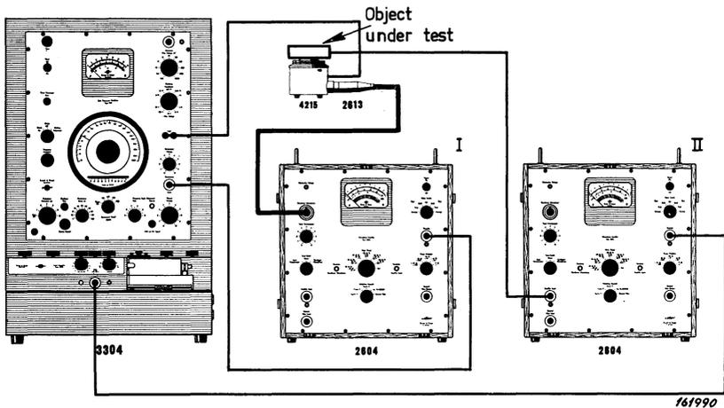
Fig. 12. Measuring arrangement for recording the frequency response of small microphones.
