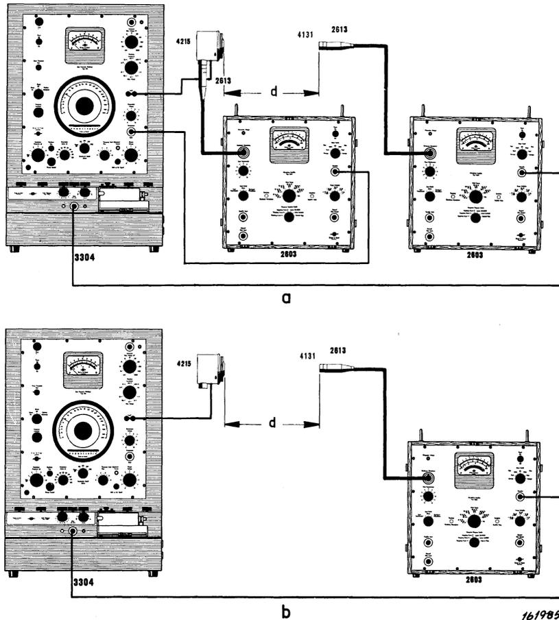
Fig. 7. Measuring arrangements used to obtain the curves shown in Fig. 5 and 6 respectively.
