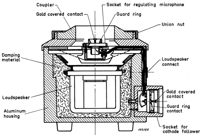
Fig. 1. Sectional view of the Artificial Voice.
