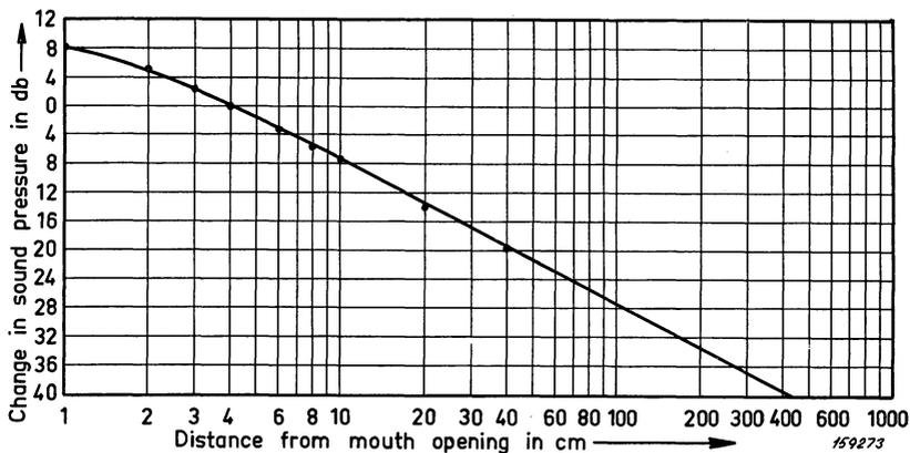
Fig. 10. The variation in sound pressure as a function of distance. Measured with a microphone which has negligible effect on the sound field.
