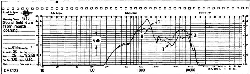
Fig. 8. Curve showing the influence of a 24 mm microphone with flat front placed in a distance of 4 cm from the mouth opening. Curve II shows the frequency response as taken with the 24 mm microphone and curve I shows the frequency response as obtained with a microphone which has negligible effect on the sound field.
