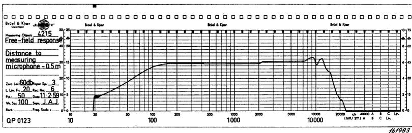
Fig. 5. Free field response of Type 4215 with regulating microphone employed.
