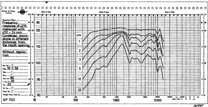
Fig. 9. The variation of the frequency response with distance when measuring the nearfield with the above mentioned 24 mm microphone.
