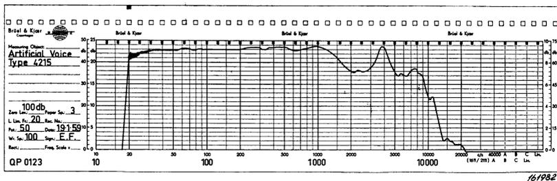
Fig. 4. Pressure response curve of 4215 without regulation (regulating microphone inserted but not used for regulation).
