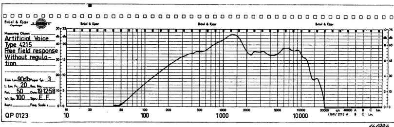
Fig. 6. Free field response without regulation (microphone inserted, but not employed).
